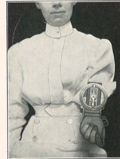
FIG. 2.—Pronometer. Indicator points to 90 degrees when forearm is in "mid-pronation."
